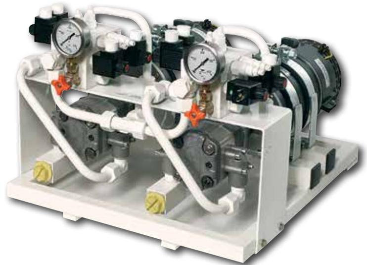
Sailing yacht power systems typically include one or several generator mounted hydraulic pumps and in addition will require a DC power pack for silent sailing and light maneuvering. The PowerValve™ power pack range used in our systems, offers exceptional flexibility and power efficiency over a wide range of hydraulic flows.
